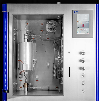
Flow Reactor (FR-100) Interior
