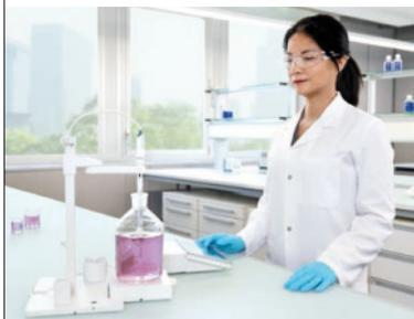
The EasyMix™ magnetic stirrer homogenizes samples for more accurate results. Its perfect fit with the EasyPlace™ electrode arm saves bench space.
