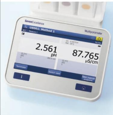
The instrument gives you the choice! By a single keypress you can switch between two different views with varying degrees of information. In the uFocus™ view, you will not be distracted by information that is of less importance.
