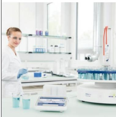
With the flexible InMotion auto-samplers, automated calibration of sensors and measurements up to 300 samples are possible. Professional automation ensures security and comfort at maximum efficiency.
