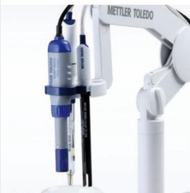
SevenExcellence allows for measurements of 1, 2 or 3 parameters simultaneously, either in the same or different samples. With multi-channel measurements the temperature signal from one module can be used for all others to ensure identical temperature readings!
