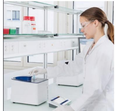
The UV5Nano combines two instruments in one for micro-volume and cuvette based measurements. Once the arm is at a 90 degree position, the measurement surface can be easily accessed with a pipette from either the left or the right. The curved lid on top of the instrument allows convenient positioning of the operator's hand to securely guide the pipette tip.
