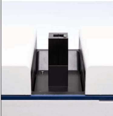
Thanks to the FastTrack UV/VIS technology, there are no moving parts in the instrument, and thus it reduces the risk of misalignment. This not only contributes to accuracy, not also brings a low requirement of maintenance.
