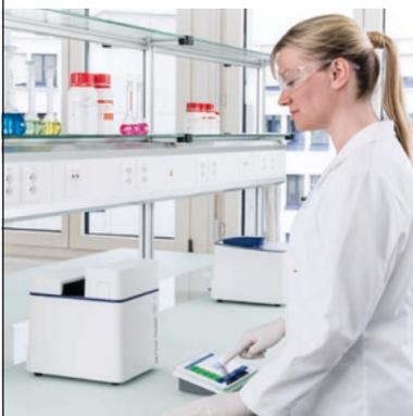
The fully automatic modules CertiRef™ and LinSet™ allow to test the performance of the instrument in compliance with Pharmacopeia (USP or Ph.Eur.). Certified reference materials traceable to NIST primary standards are used and a report documents all results. Performance verification has never been so easy, efficient and secure.
