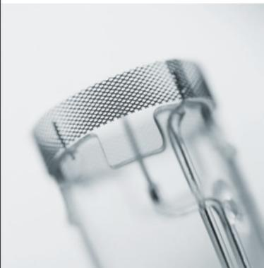
Handling of different reagents for catholyte and anolyte can be complicated and expensive. For most samples the generator cell without diaphragm offers more convenience in use. No catholyte is needed and the anolyte can be exchanged with the Solvent Manager on One Click<sup>®</sup>. Only a few samples still require a cell with diaphragm, which is clearly explained in the METTLER TOLEDO applications brochure.
