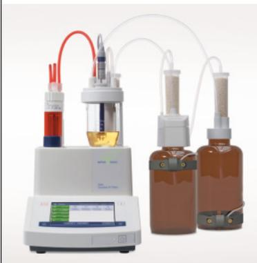
Contact with Karl Fischer reagents should always be avoided. The Solvent Manager takes care of filling, draining and exchange of the reagents. It is fully controlled by the titrator which offers One Click access to all tasks. LevelSens additionally increases security by monitoring solution and preventing overflow in the waste bottle.
