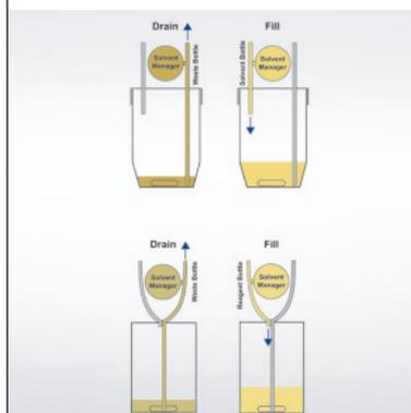
The solvent needs to be replaced regularly in order to guarantee consistently correct results. The Solvent Control supports the user by monitoring different parameters. Even when an instrument is running on Standby the Solvent Control is active and automatically starts conditioning of the fresh solvent after exchange. With minor user interaction the system is always kept in optimum condition ready to ensure a quick, accurate result whenever required.
