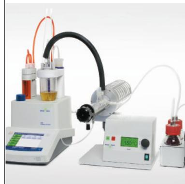
METTLER TOLEDO's D0308 drying oven allows safe and easy oven application for single samples. The manual oven D0308 assures accurate water determination combined with simple handling.
