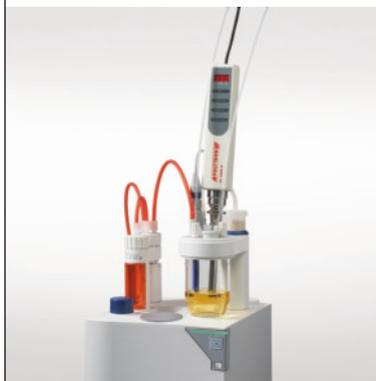
Solid samples which do not dissolve in the Karl Fischer solvent can be added to the titration vessel and ground with a Homogenizer. The Homogenizer speed is controlled by the Excellence titrator via the RS-interface and documented. This guarantees maximum security and full GLP-compliance. Special chemicals for extraction are avoided using the Homogenizer for grinding.
