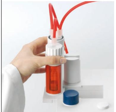
Automatic burette recognition feature ensures that all quality-relevant data such as concentration, titer and expiration date are promptly read in and checked, irrespective of the drives on which the burettes with the titrants are present. The password-protected user management system coupled with user rights guarantees that critical data cannot be changed by mistake.
